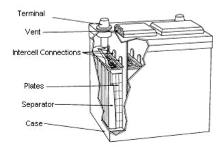
Eighty percent of all battery failure is related to sulfating build-up. This build-up occurs when the sulfur molecules in the electrolyte (battery acid) become so deeply discharged that they begin to coat the battery's lead plates, and before long, the plates become so coated the battery dies. The causes of sulfating are numerous:
