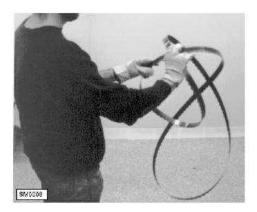
See Figure 4-6. Keeping the blade in its crossed position, take hold of the side crossed UNDER with your other hand. Use your right (or left) hand to hold only the side crossed OVER. Place your thumbs on the top side of the blade. Put your fingers on the underneath side of the blade.
