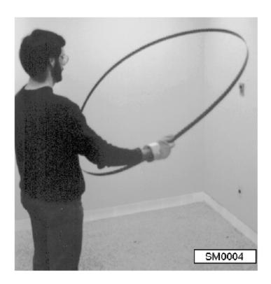
See Figure 4-2. Keeping your wrists locked in position, turn your forearms upward and inward. (The teeth will rotate inward and the bottom of the blade will rotate outward.)
