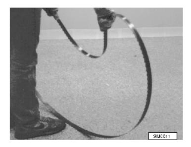
See Figure 4-10. Keeping your hands close together, rotate the curved section of the blade up and away from you. The blade will be in an oval shape, but twisted.
